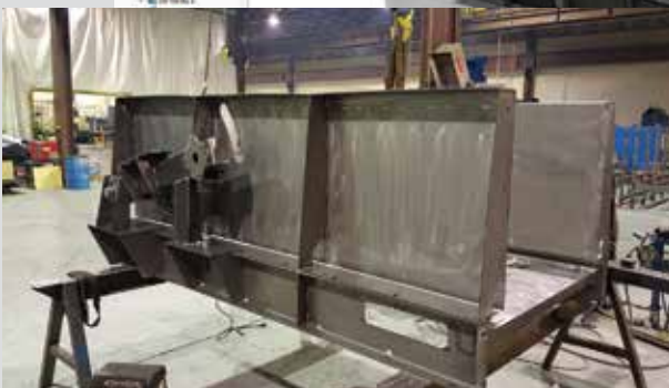
Conveyor Section with Custom Metering Wheel
